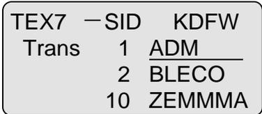
5. PRESS **ENT** to view the waypoints of the SID and provide the option which allows you to add it to the flight plan.
