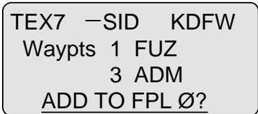
6. PRESS **ENT** to load into flight plan. The first waypoint of the SID automatically becomes the active waypoint.
